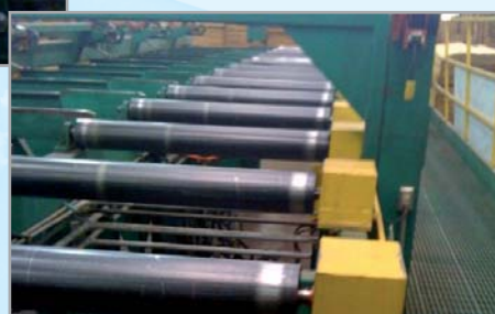
Roller conveyors with BEHAbelt Round belts PU 85 A PLUS
