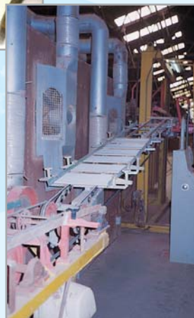
Tile conveying via BEHAbelt pointed V-belts PU 90 A, profile C, 22 x 24 mm
